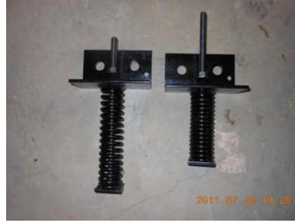
6) If the floor joists are perpendicular to the wall, secure the top of the beam using the stabilizer strap. Place the top bracket (spring Side) against the face of the beam and mark the two holes in the bracket. Remove the bracket and drill out the holes through the floor joists. Try to keep the holes near the center of the joists. Bolt the top bracket in place. **Repeat these steps for all locations before releasing the spring pressure.**
